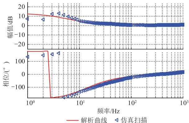
图 3 风电机组  $d$  轴阻抗解析曲线与仿真对比Fig.3 Comparison of theory curve and simulation of D-PMSG  $d$  axis impedance
