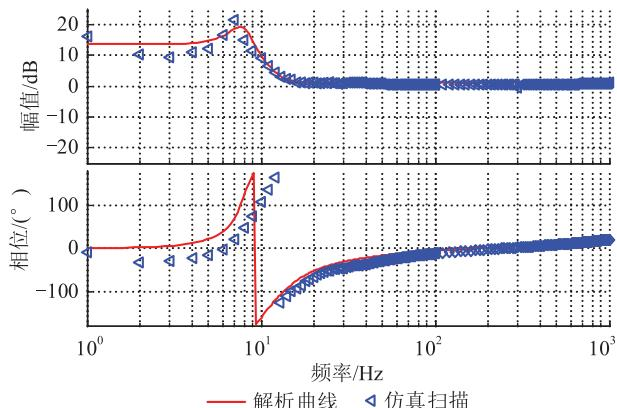
图 4 风电机组  $q$  轴阻抗解析曲线与仿真对比Fig.4 Comparison of theory curve and simulation of D-PMSG  $q$  axis impedance
