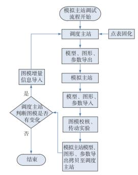
图 2 基于模拟主站的变电站信息接入调试流程示意图 Fig.2 Schematic diagram of substation information access debugging based on simulation master station
