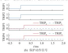
图 12 末端经过渡电阻正极故障动作特性 Fig.12 The action characteristics of terminal positive electrode fault through transition resistance
