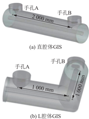
图6 GIS各特高频传感器校验模型 Fig.6 GIS model for each ultra-high frequency sensor verification
